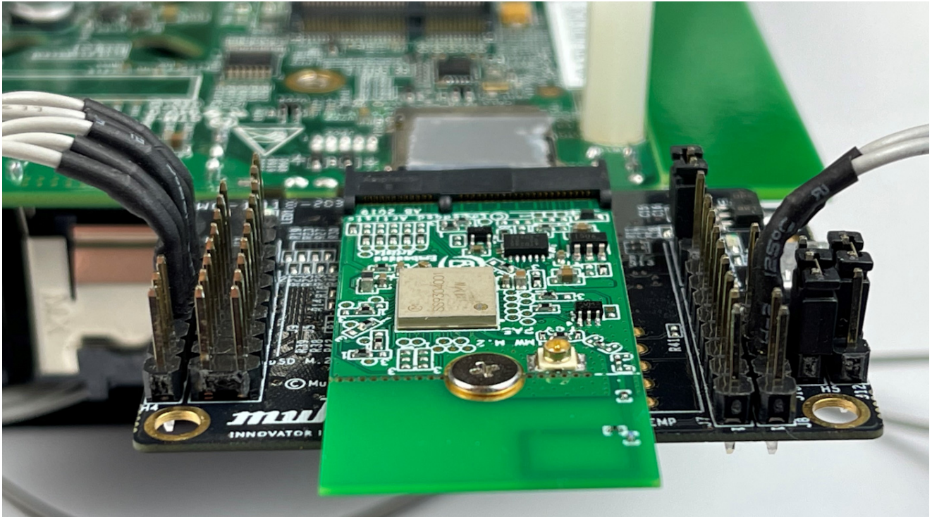
Figure 45: Low-Profile Jumper Wires (Digi-Key part number 1988-1178-ND)
