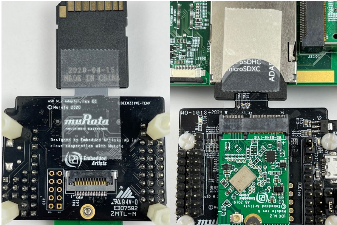
Figure 16: Securing uSD/SD Connection on i.MX 6 EVK
