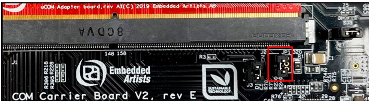
Figure 5: J2 jumper (closed for flashing mode) on Developer's Kit
