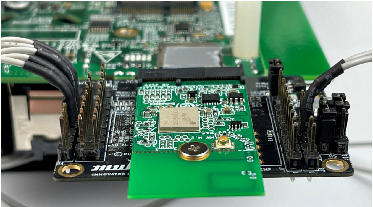
Figure 24: Low-Profile Jumper Wires (Digi-Key part number 1988-1178-ND)
