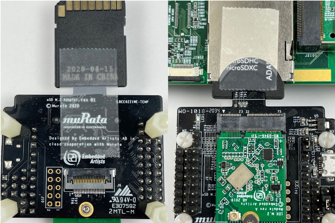
Figure 29: Securing uSD/SD Connection on i.MX 6 EVK
