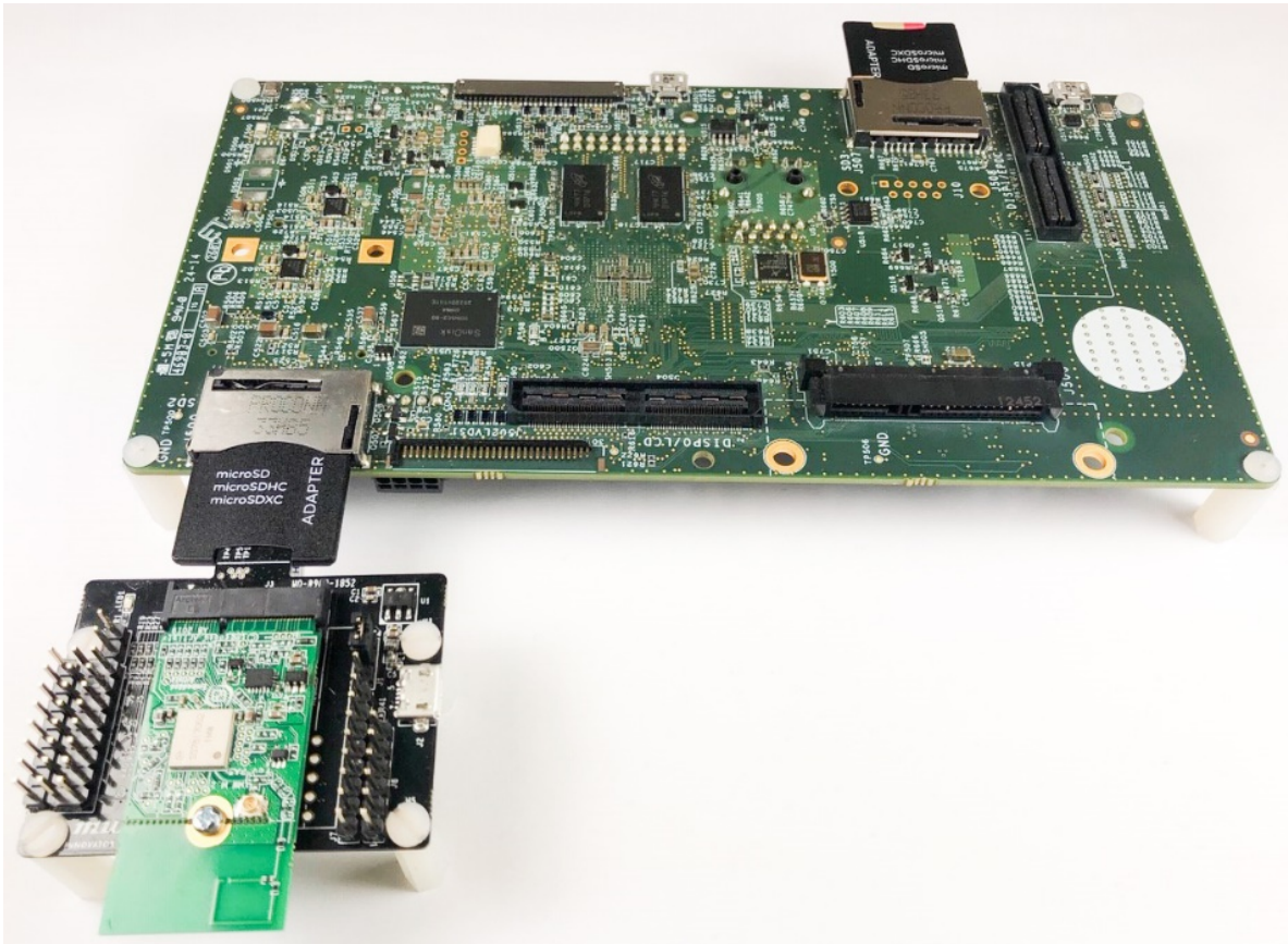
Figure 14: i.MX 6Quad/DualLite SDB (Inverted) with uSD-M.2 Adapter and Type 1MW M.2 EVB
